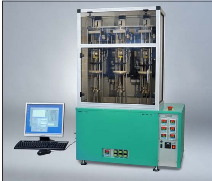
Test station for testing in compression and for testing in tension.
