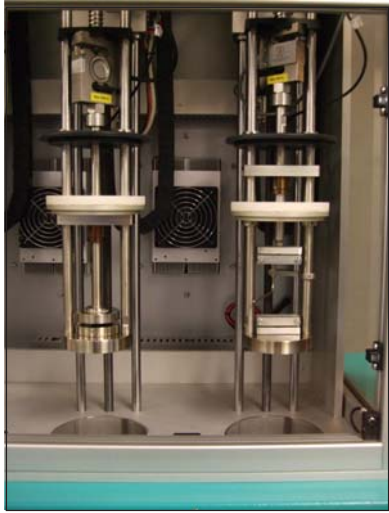
Test station for testing in compression and for testing in tension.
