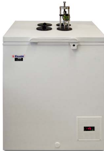
The test rig in the Freezer ET03 adapted for Low Temperature compression set.
