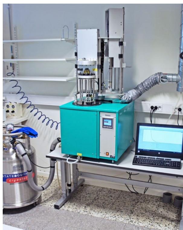
Combined low temperature instrument with a Gehman tester (ET 02-II) selected, placed on the adjustable table ET 01.08.
