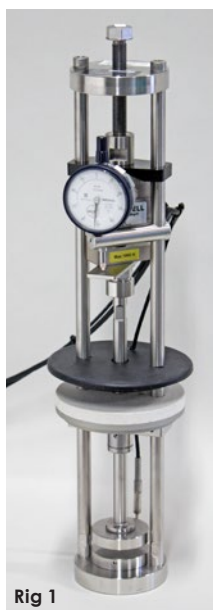
Rig 1 is arranged for testing in compression according to ISO 3384 and ASTM D6147.
