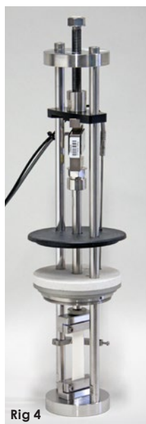
Rig 4 is arranged for testing in tension according to ISO 6914 method A.
