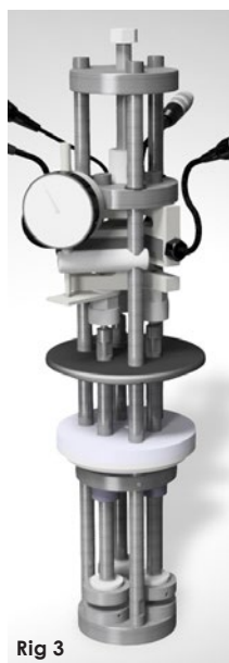
Rig 3 is a triple rig for compression according to ISO 3384 and ASTM D6147.
