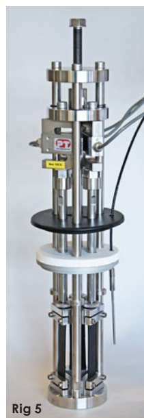
Rig 5 is a triple rig for tension according to ISO 6914 method A.
