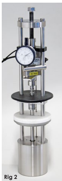
Rig 2 is arranged for testing in liquid according to ISO 3384.
