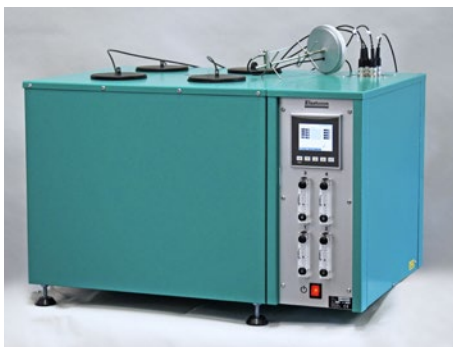
The EB 19 cell oven is equipped with 4 cells, each with individual flow meters and individual temperatures.
