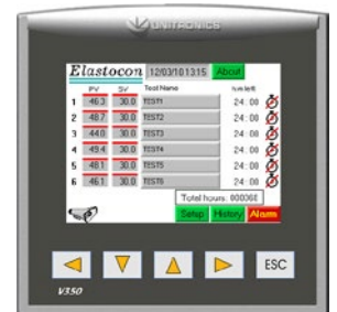
All ageing ovens are controlled from a colour touch screen.
