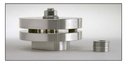
Compression Set Rig, EV 03, according to ISO 815. The rig consists of two circular polished plates of stainless steel with a central screw and spacer. Designed to be suitable for holding in a conventional vice to aid sample loading, the rig utilises the minimum of components. Spacers for both small and large test pieces are included.
