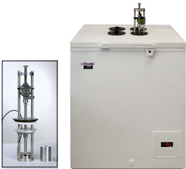
Figure 19, Automatic Low Temperature Compression Set tester
