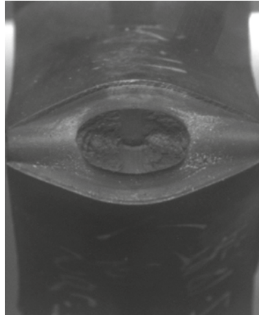
Crack growth after 100.000 samples at 60°C
