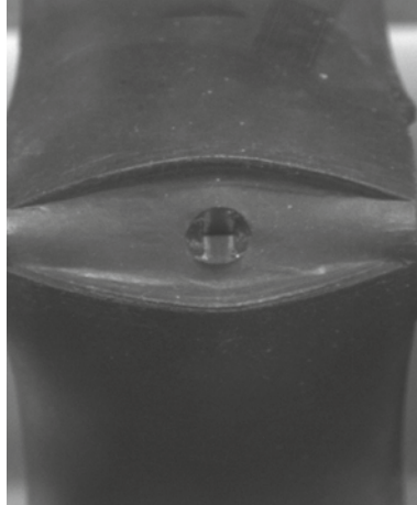
Automatic image recording by CCD Camera Initial, pierced sample acc. ISO 132
