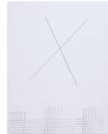
Aluminum panel made from alloy X shows excellent paint adhesion
