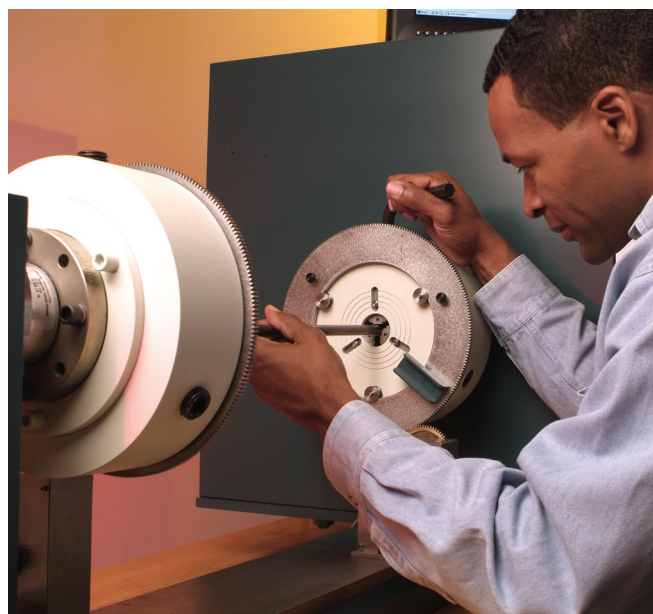
Samples are easily mounted in the patented bidirectional grips.
